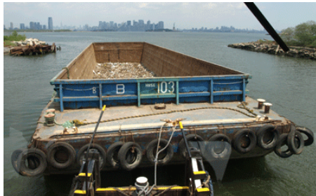
Pushing straight through the opening and setting up for the next 90 degree turn to port. Note the slack in the line. I am letting the boat drift along behind the barge to allow the barge to slow down.
