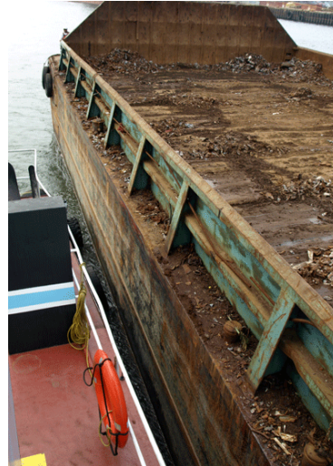
Alongside a light scrap barge with the Herbert Brake. Just a headline is out on the forward quarter bitt
