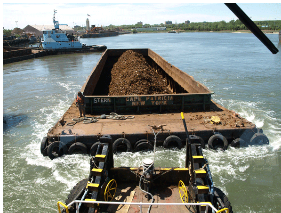
Backing a hopper loaded with 1,500 tons of shredded steel drawing 15 ft ¼ mile from the barge racks to shipside. This barge move takes 35 minutes on push wires but only 20 minutes on one line.
