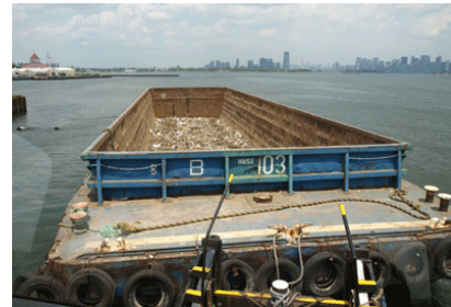
Beginning the turn. The boat is angling off to starboard and pushing the bow around to port, as well as, ahead.
