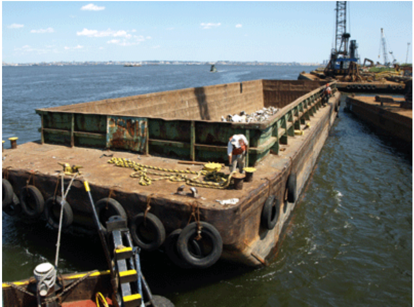
Backing a barge over to another barge – just keep the headline pointing in the way that you want the barge to go.
